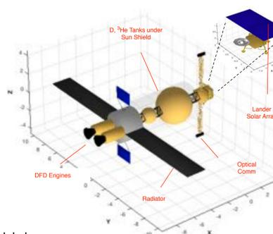
The MATLAB model shows estimated sizes for the fuel tanks, radiators, and lander solar array for receiving power.
