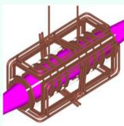
RF frequency power (0.2 to 4 MHz) is applied by antennas outside the plasma vessel.
