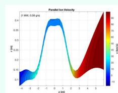
Propellant heating is modeled by the UEDGE fluid code to study thrust and specific impulse of rocket operation.
