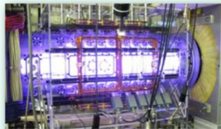
Neutrons are reduced through choice of fuels (D-<sup>3</sup>He), fuel ratio (D:<sup>3</sup>He = 1:3), and machine size. Tritium, a byproduct of D-D fusion, is exhausted before it can fuse.
