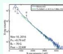
X-ray spectra on the experiment indicate electron temperatures exceeding 500 eV with 20 kW input power
